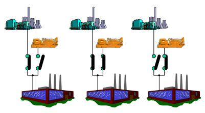
The closed transition transfer switch waits until the two sources are "synced".
