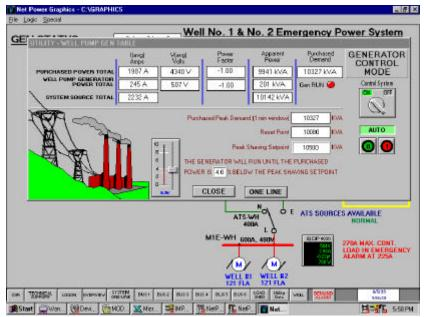
Figure 2: Screen shot showing incoming campus demand, settings for when generator is to automatically start and when it is to automatically disengage.
