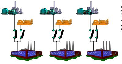
The open transition transfer removes power to the load when it switches from one source to another.
